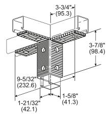
FITTING DATA: Each fitting 1/4" thick, 15/8" wide • Holes 9/16" diameter, centered 17/8" apart, 13/16" from edge
