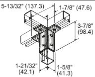
FITTING DATA: Each fitting 1/4" thick, 15/6" wide • Holes 9/16" diameter, centered 17/6" apart, 13/16" from edge
