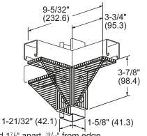
FITTING DATA: Each fitting 1/4" thick, 15/6" wide • Holes 9/16" diameter, centered 17/6" apart, 13/16" from edge
