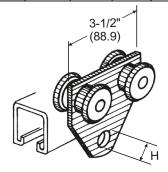
Allowable load 600 lbs (2.67 kN) maximum. Trolley designed to fit N-200 and N-210 channels.
