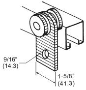
Allowable load 300 lbs (1.48 kN) maximum. Trolley designed to fit N-200 and N-210 channels.
